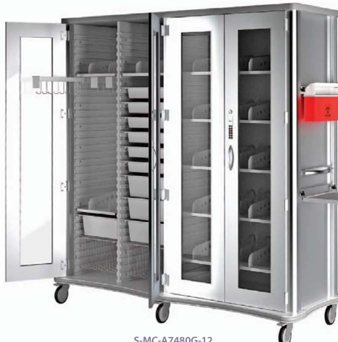
S-MC-A7480G-12 29-1/2"D x 74"W x 80"H 6 - 4" tray with 3 short and 3 long dividers 4 - 6" tray with 2 short and 2 long dividers 2 - 10" wire basket 13 - 24" metal shelf 26 - 24" adjustable metal shelf dividers 3 - 9" inline hook cath manager Roll top model S-MC-A7480-12 Shown with optional accessories (Sold separately)
